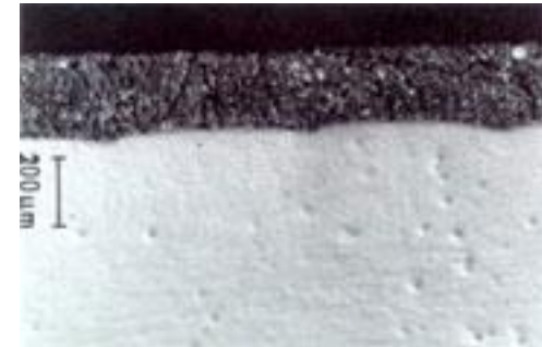
Cr 2 O 3 coating with a thickness of ca. 200 μm, deposited using a CO 2 laser and treated with a Nd-YAG laser.
