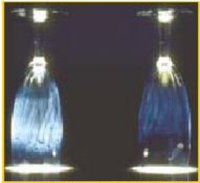
'Milky' wineglass (left) and how it should look (right). (Courtesy of Himanshu Jain.)
